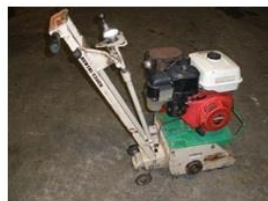
Edco CDM 8 Line Removal Grinder
