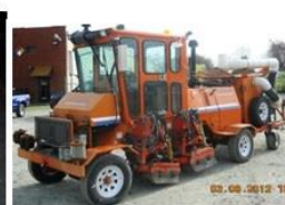
2008 Swanston CT 2000 Line Removal Grinder with Vacuum,
